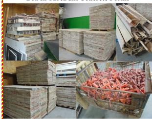
13 Pallets of Concrete Forms 2x4 (40) forms per pallet = 520 linear ft of wall - approx.), 6 Pallets of Concrete Forms 2x8 (40 forms per pallet - 240 linear ft of wall - approx.), Corners, Fillers & Hardware
